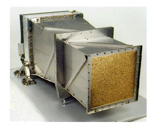
Wide X-ray FOV  $\rightarrow$  traditional optics not applicable because X-rays can only be reflected at grazing angle of less than 1 degree. Alternative: coded aperture imaging principle
