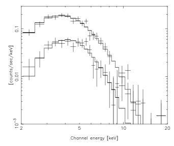
**Fig. 5.** Spectra of the 71 s lower-flux interval (lower spectrum; first interval between vertical lines in Fig. 4) and the 41 s interval after the dip (upper spectrum; last interval in Fig. 4). The crosses indicate the measurements (vertical lengths indicate  $1\sigma$  error intervals; histograms indicate the fitted model with free  $N_{\rm H}$  and fixed radius).
